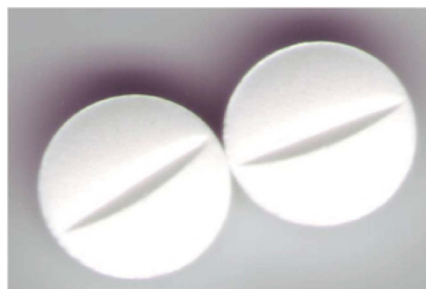
Figure 2. Examples of compressed tablets. Their shape is biconvex with straight-through bisect and their diameter is approximately 6.35 mm.
